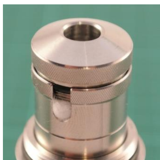
Pic 14: Screw the chamber cap onto the chamber sleeve and tighten carefully.
