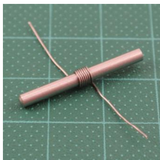
Pic 2: Create a coil. The wire ends should point in the opposite direction.
