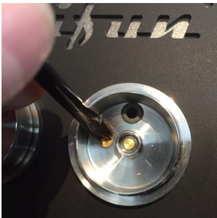
Step 7: Clean the sensor completely with a water-soaked brush and then pat dry again. The chamber should now be clean again.
