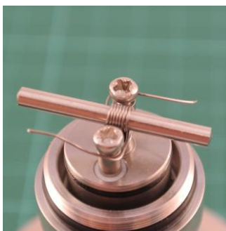
Pic 3: Install the coil as centrally as possible between the two poles.
