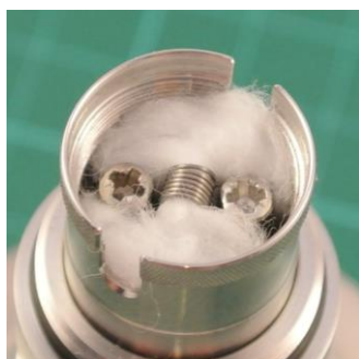
Pic 13: The cotton should now fit the chamber well. Now, you can pre-moisten the cotton with a suitable liquid.
