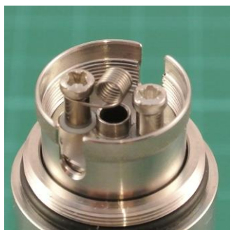
Pic 9: Now push the chamber sleeve down, until it clicks into place.
