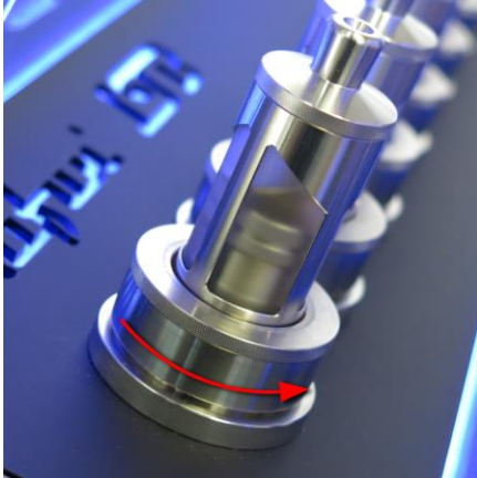
Step 1: The sealing ring is unscrewed counterclockwise.
