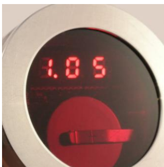
Pic 7: Check the resistance using an appropriate meter (e.g. Taifun® Omega).
