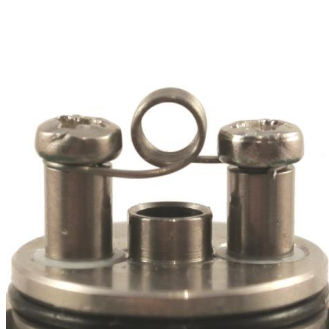
Pic 6: The coil should be located centrally between the poles.
