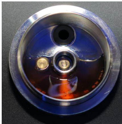
Step 5: Now you should check if liquid is in the connection chamber.
