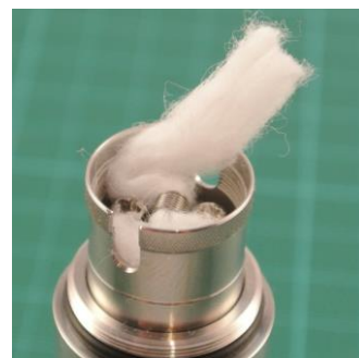
Pic 12: Arrange the cotton in the chamber (S-shape).
