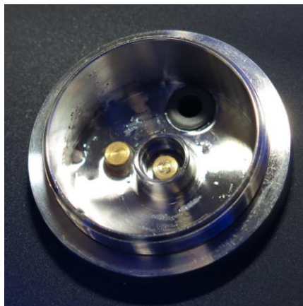
Step 8: After cleaning it may be necessary to put saline solution into the chamber, again. Now, the atomizer can be screwed on.
