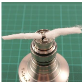
Pic 10: Guide the cotton through the coil..
