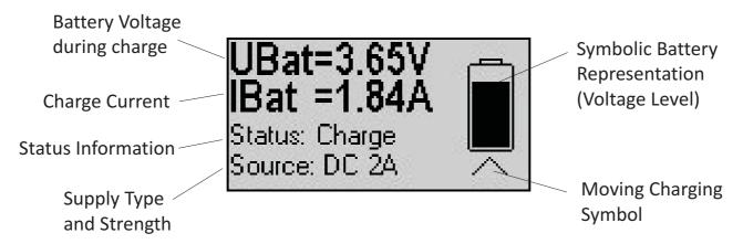
On the left side of the display, the permanently updated parameters of UBat (battery voltage level) and IBat (charging current) are shown. Below this, the identified source and its strength as well as the current operation status is displayed.
